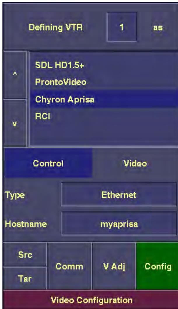
Figure 5. Video Configuration Panel with Aprisa DDR set-ups.
