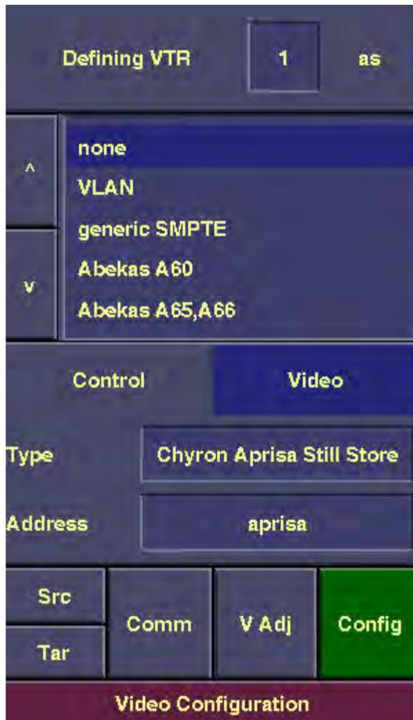
Figure 11b. Video Configuration panel set up for Aprisa Still Store
