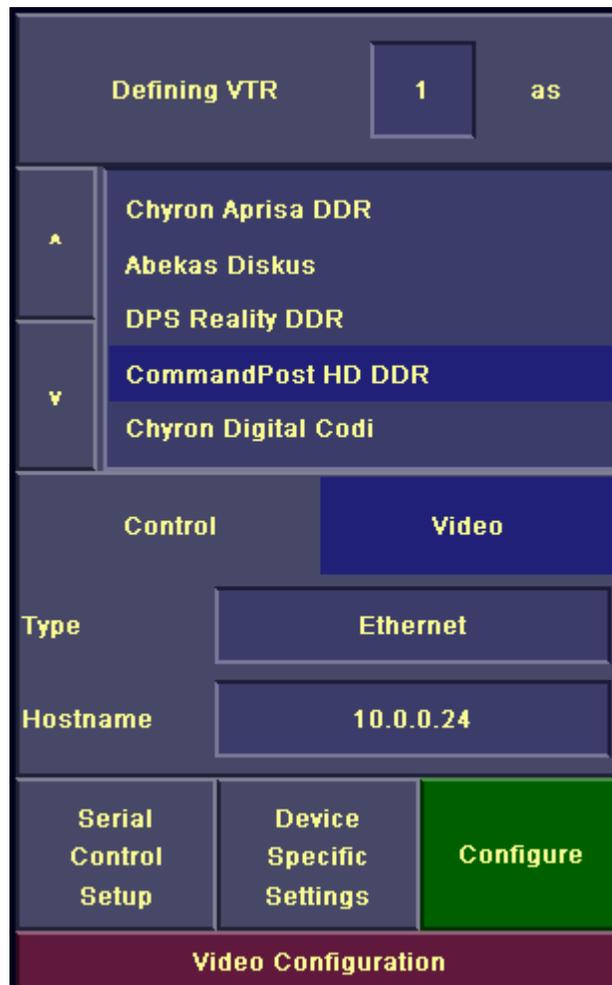
Figure 2.1 – Video Configuration Panel configured for CP HD DDR.
